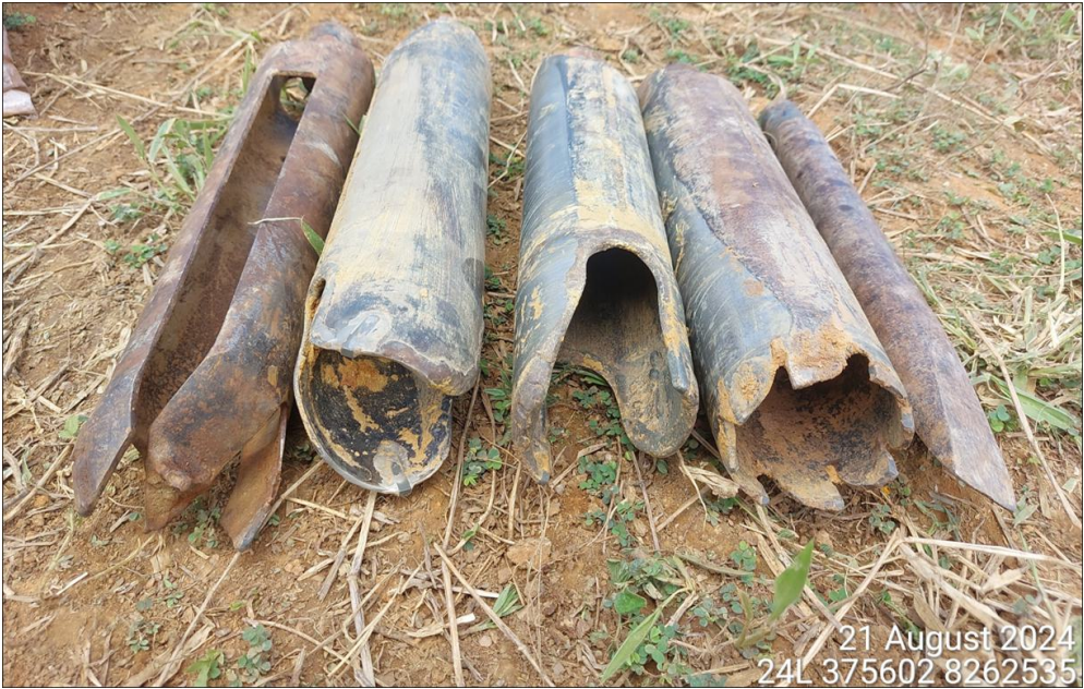
Figure 7-5 Auger coring blades (from left, used for soils coring, conventional coring, for harder substrate, for clays, rock breaker)
