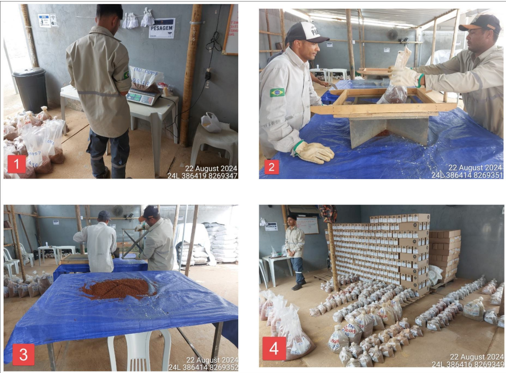
Figure 8-1 Sample preparation at Itarantim sample yard – (1) weighing sample; (2) screening and quartering of sample; (3) quartered sample; (4) sample bags ready for distribution, returned pulps in boxes
